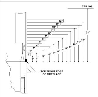
Figure 28. **Minimum Vertical and Maximum Horizontal Dimensions of Combustibles above Fireplace**
